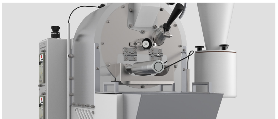
Large pyrex lens for easy monitoring, beans temp probe
