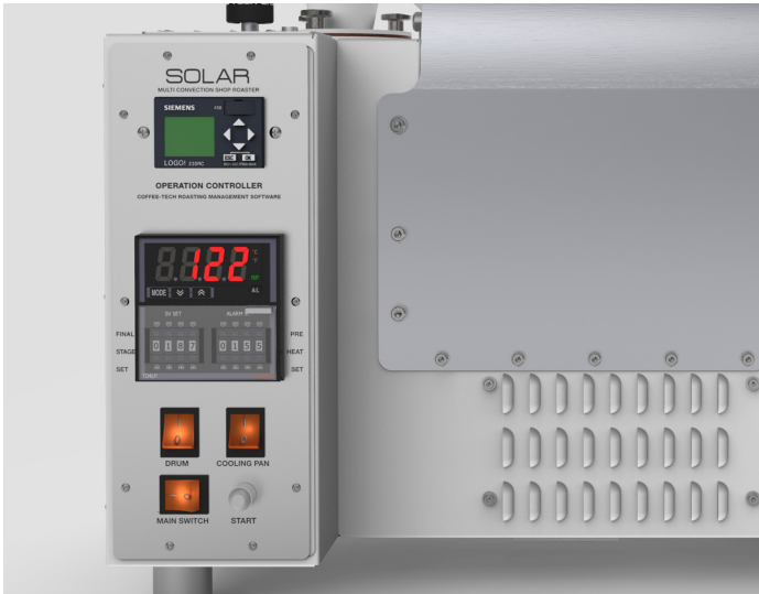
Panel de Control →
